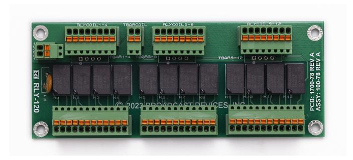
The RLY-120 Relay Interface panel provides a way to take a single closure to control up to 12 relays simultaneously. In addition there is provision to program the panel to accept individual relay commands where the coils of each relay are brought out to terminal blocks. Relay outs are also brought out to convenient pluggable terminals.
